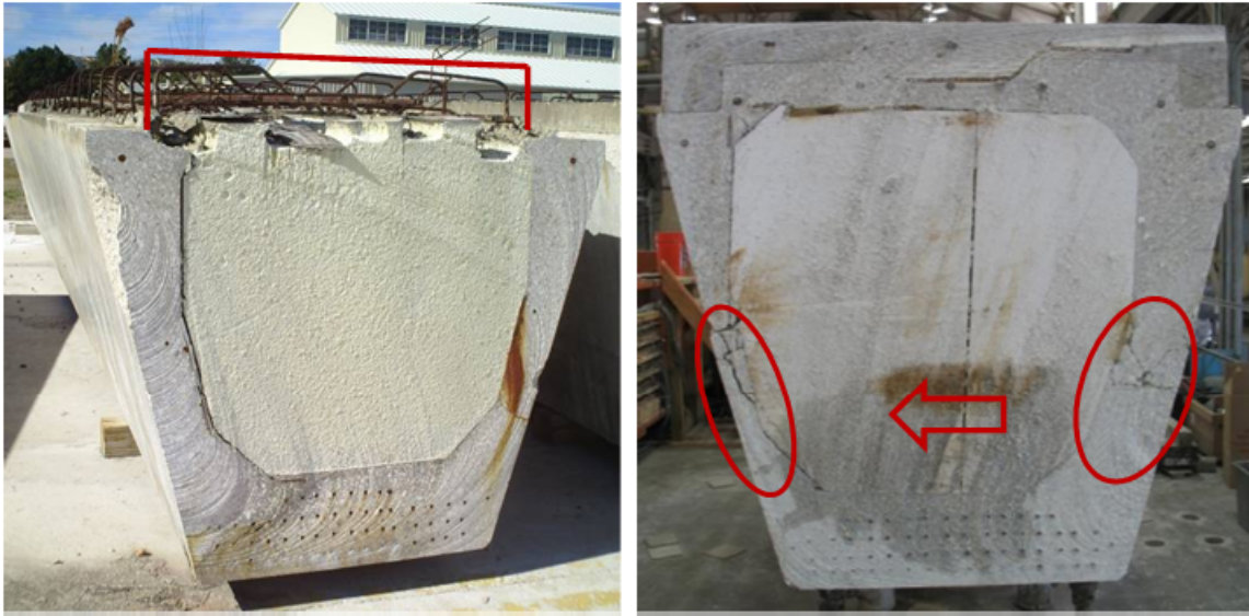
Figure 3-7: Examples of Vertical and Horizontal Void Misalignment
