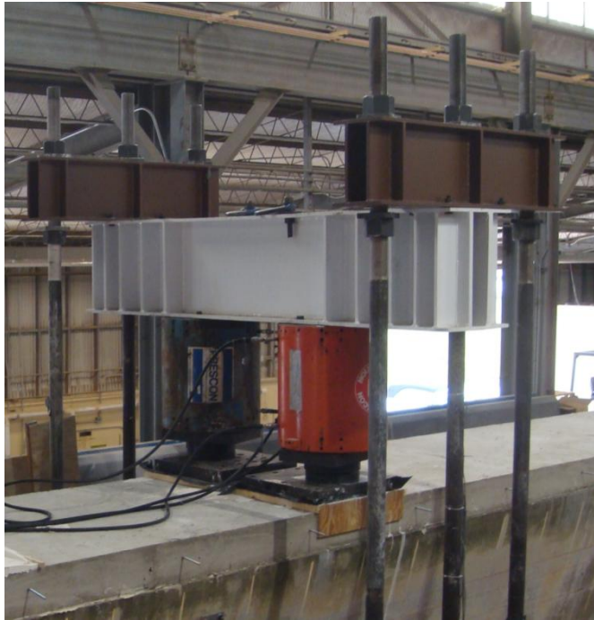
Figure 3-17: Four-Million Pound Loading Apparatus
