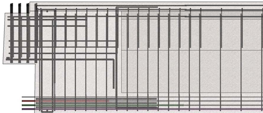
(C) Typical Dapped End Reinforcement Layout
