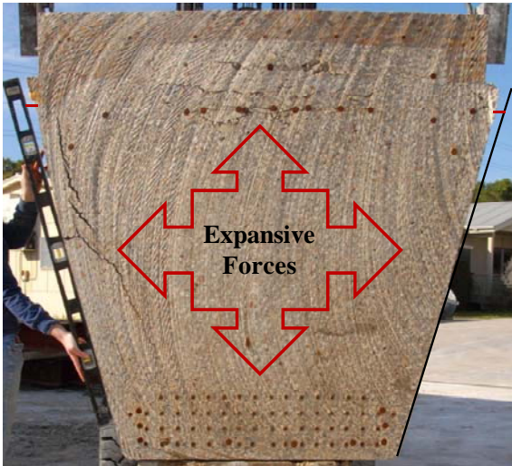
(C) Distortion of the Cross-Section Geometry
