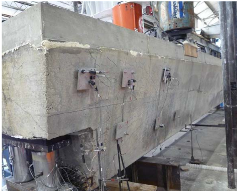
Figure 3-23: L-II Fully Instrumented for Dapped-End Testing
